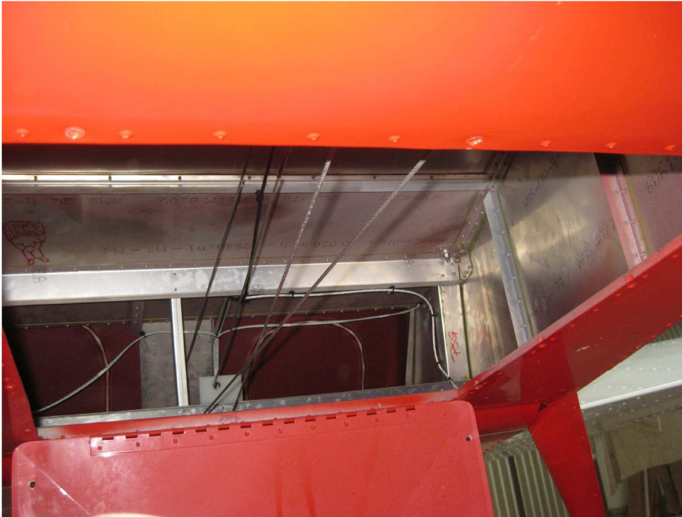
Below: Turn-buckles to be used if cable tension needs to be adjusted.
