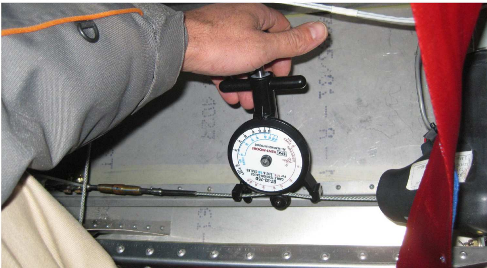
Photo of tensiometer on left Aileron cable seen from pilot seat (see flap motor on right). Repeat process on right aileron cable, behind passenger seat.
