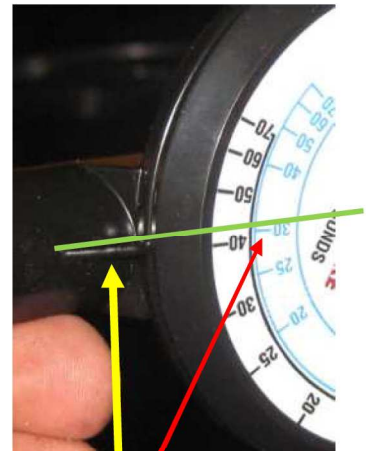
Index mark (read blue scale for 1/8 cables)
