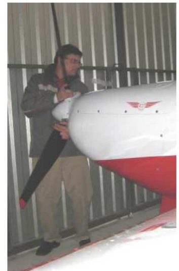
Have nose wheel lifted off the ground while rudder cable tension is checked. (no necessary with tail dragger)
