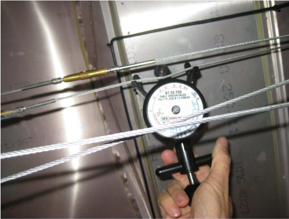
Above: Checking elevator cable tension inside fuselage.
