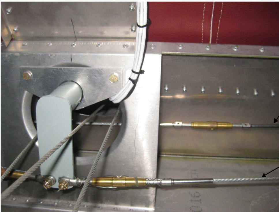
Note the aileron turn-buckle for the “balance cable” (forward of the right aileron cable in the background of this photo)
