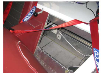
The aileron cables can easily be reached from the cabin area, behind seat backs.
