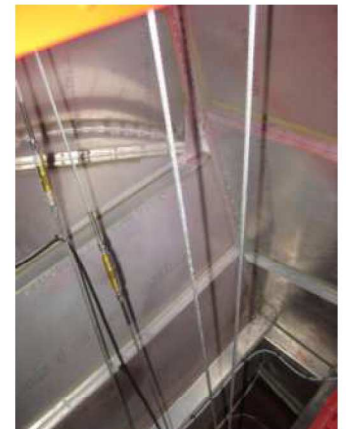
If fuselage door not installed, elevator cable tension can be measured through access holes behind seat backs.
