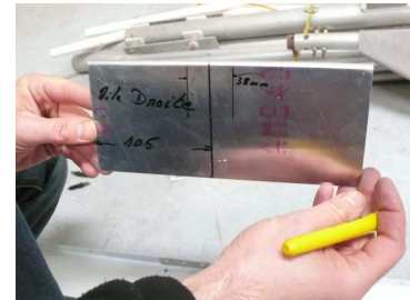
Mark a center line on the Aileron Rod Hole Doubler (6Z-2G-2)
