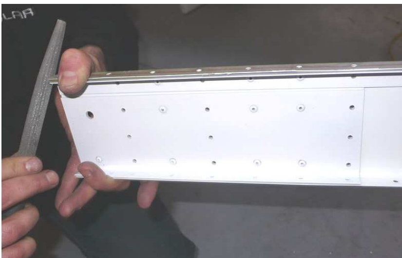
After setting rivets, remove any remaining burrs or sharp edges; then paint to match rest of wings.
