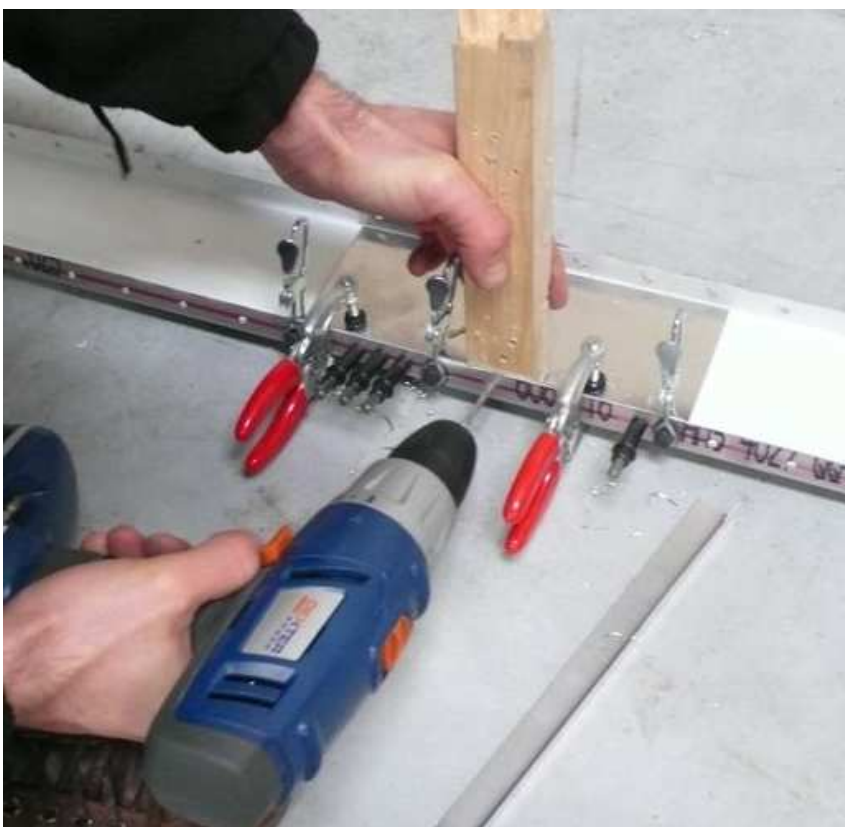
Back-drill holes along flange. Cleco in place.
