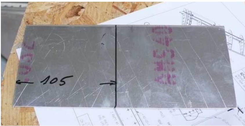
Mark a center line on the Aileron Rod Hole Doubler (6Z-2G-2)
