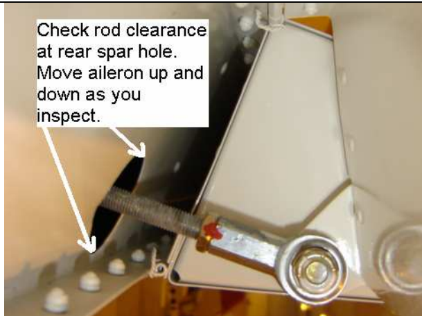
View of aileron, from bottom of wing area
