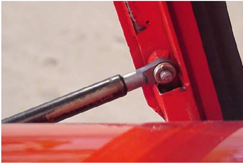
283. Canopy gas strut installation with cotter pins. 601 XL and 650
